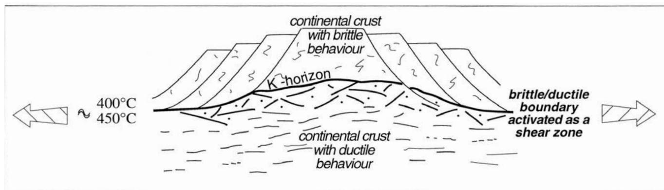
Fig. 9 - Structural interpretation of reflectivity, hypocentral distribution and temperature in the Larderello and Monte Amiata geothermal fields. (after Cameli et al., 1993).
