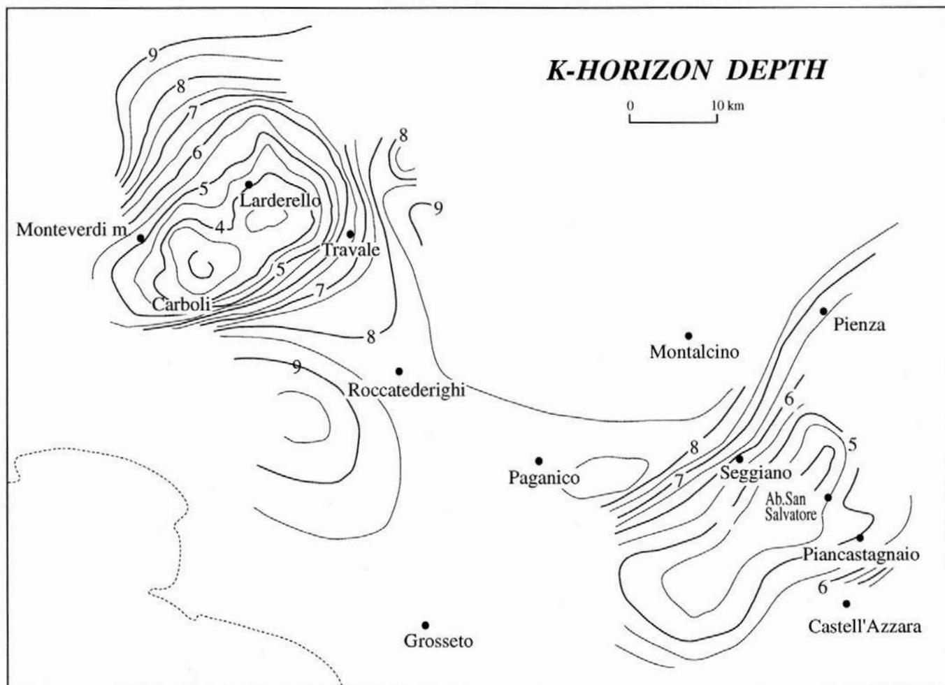
Fig. 10 - Contour lines in kilometers (interval: 0.5 km) of the depth of the K-horizon based on seismic reflection lines acquired in Southern Tuscany (after Cameli et al., 1998).
