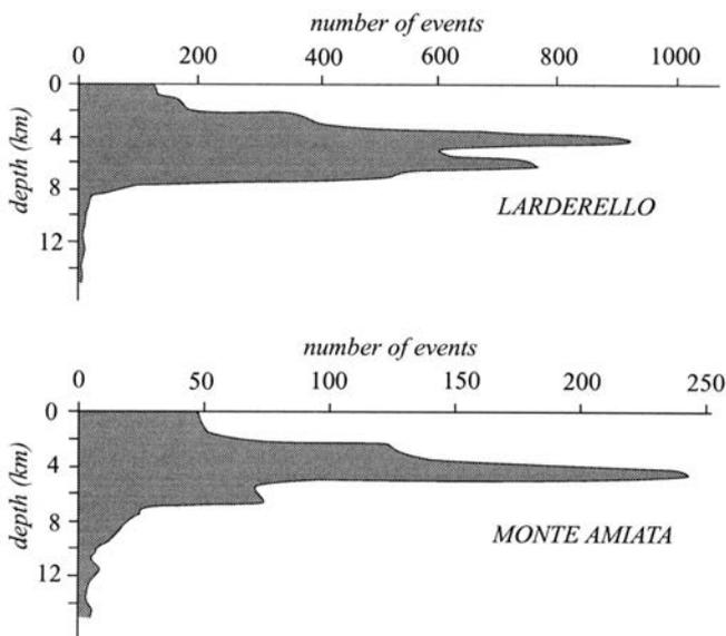
Fig. 7 - Distribution with depth of the hypocenters of local seismic events recorded by the seismic network of the Larderello (26 stations) and Monte Amiata (12 stations) geothermal fields. Larderello geothermal field: 3745 events (Magnitude  $\geq 0.5$ ) occurring in the period 1977-1995 were considered. Monte Amiata geothermal field: 839 events (Magnitude  $\geq 0.5$ ) occurring in the period 1978-1992 were considered (after Cameli et al., 1998).
