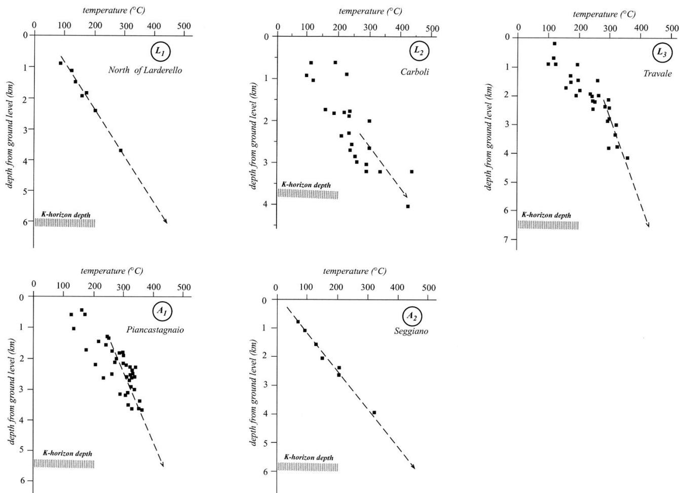
Fig. 8 - Temperatures measured in the geothermal wells of Larderello ( $L_1$ ,  $L_2$  and  $L_3$ ) and Monte Amiata ( $A_1$  and  $A_2$ ) fields. The arrow indicates the extrapolated temperature, at the depth of the K-horizon where the temperature is always ranging between 400°C and 450°C (after Cameli et al., 1998).
