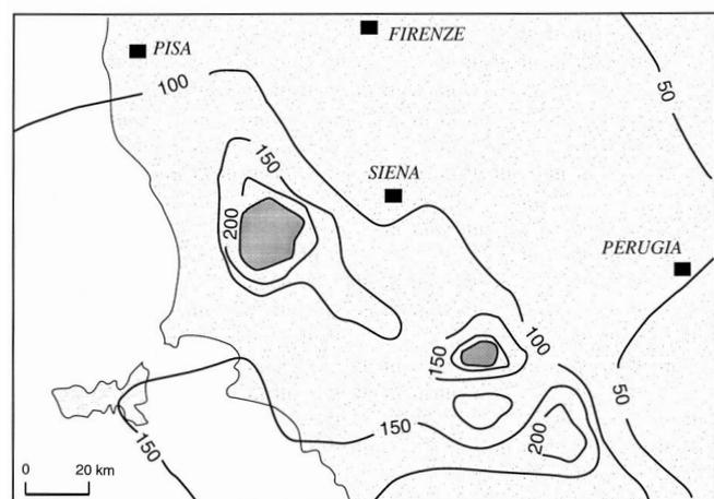
Fig. 2 - Simplified heat flow map of Southern Tuscany. Contour lines are in mW/m<sup>2</sup>. Grey areas indicate the Larderello area, to the North, and the Monte Amiata area, to the South. (after Mongelli et al., 1989 and Mongelli and Zito, 1991, modified).
