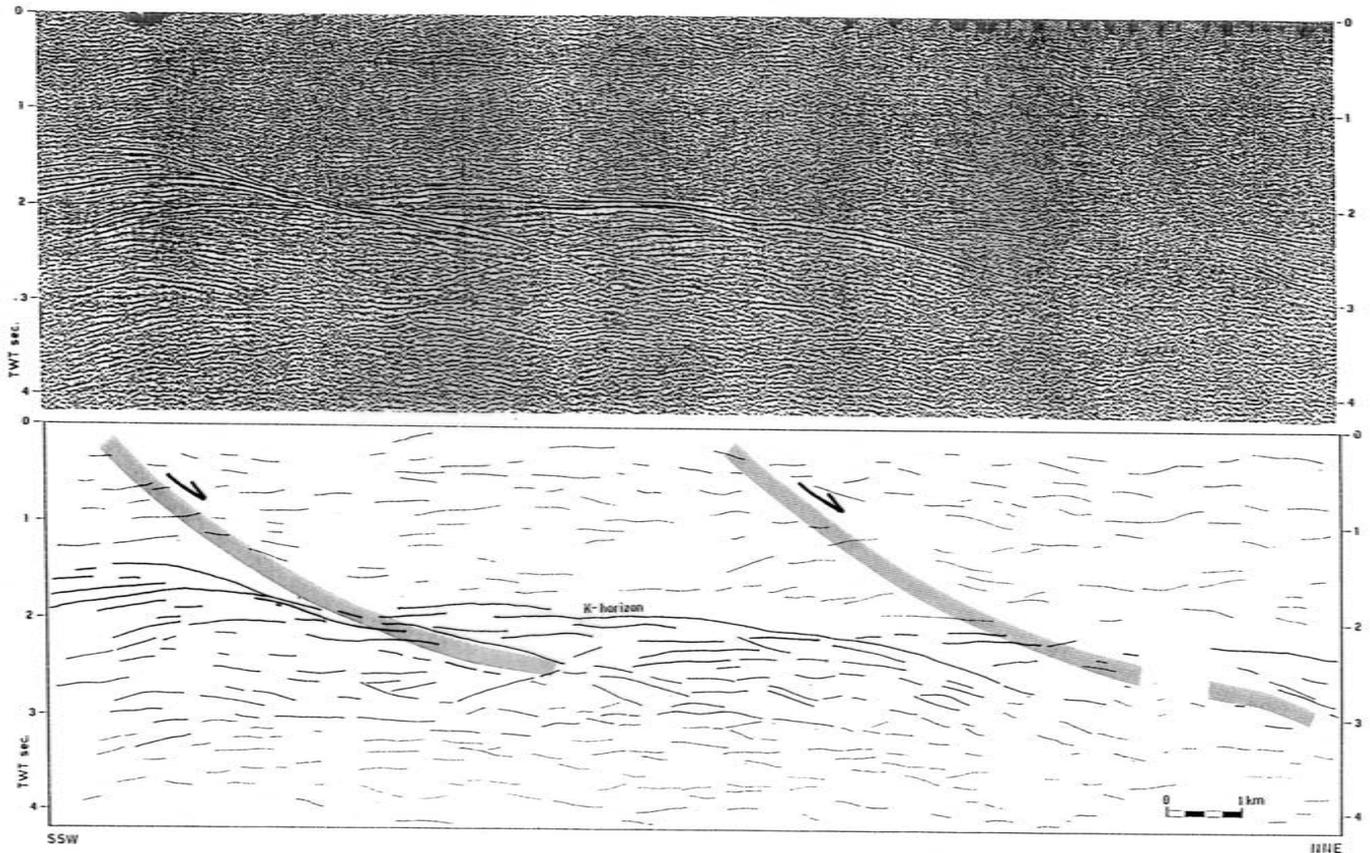
Fig. 6 - Unmigrated SSE-NNE seismic profile (top) and its line drawing (bottom) across the Larderello geothermal field. The K-horizon is affected by normal faults which are related to the third extensional event. The normal faults tend to flatten in the lozenge-shaped band (after Cameli et al., 1993, modified).
