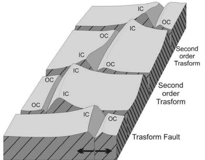
Fig. 21 - The along axis Inner Corners (IC) and Outer Corners (OC) and transform faults model for the mid-ocean ridge of the Atlantic Ocean (re-drawn after Tucholke and Lin, 1994).
