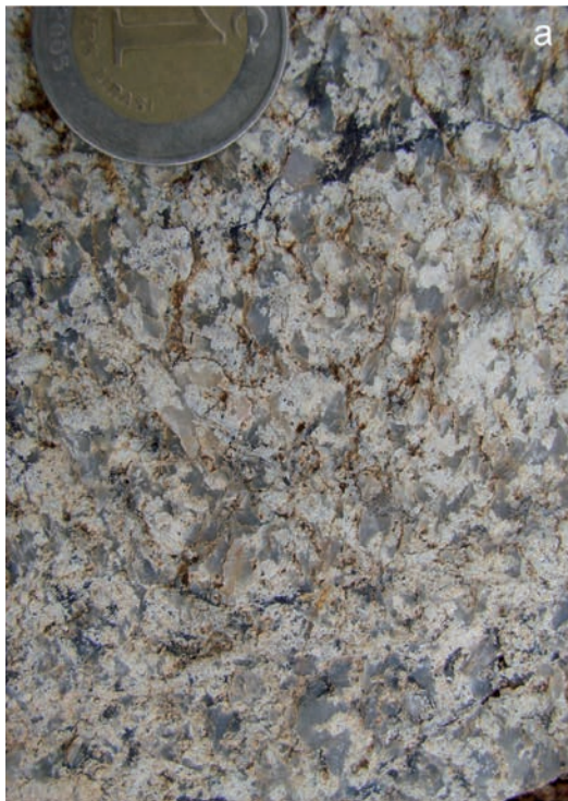
Fig. 16 - (a) Kapanca metagranitoid. The dark regions are quartz and the white regions are jadeite. (b) Single-zircon evaporation Pb-Pb ages from the Kapanca granitoid (modified from Okay et al., 2008a).
