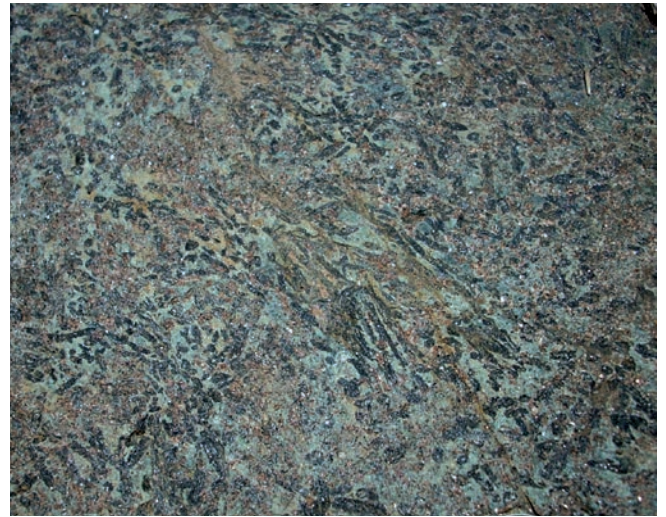
Fig. 25 - Triassic eclogite from north of Eskişehir consisting of garnet, sodic pyroxene and sodic amphibole.
