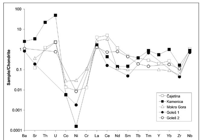
Fig. 10 - Spider diagram normalized to primordial mantle marks two processes, i) contribution of sedimentary rocks (sialic elements) in the Kamenica sample and, ii) steady decrease of Ni and Co, as well as of the Ni/Co ratio, suggesting variable degrees of weathering in the overlying lateritic crust.
