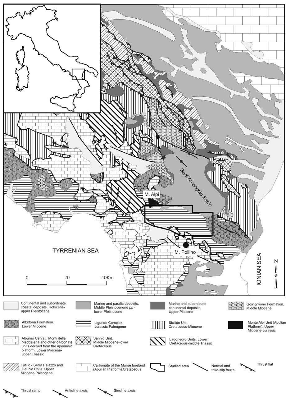
Fig. 1 - Regional geological map of the Southern Apennines; the box indicates the location of the studied area. Modified after Patacca and Scandone (2007).
