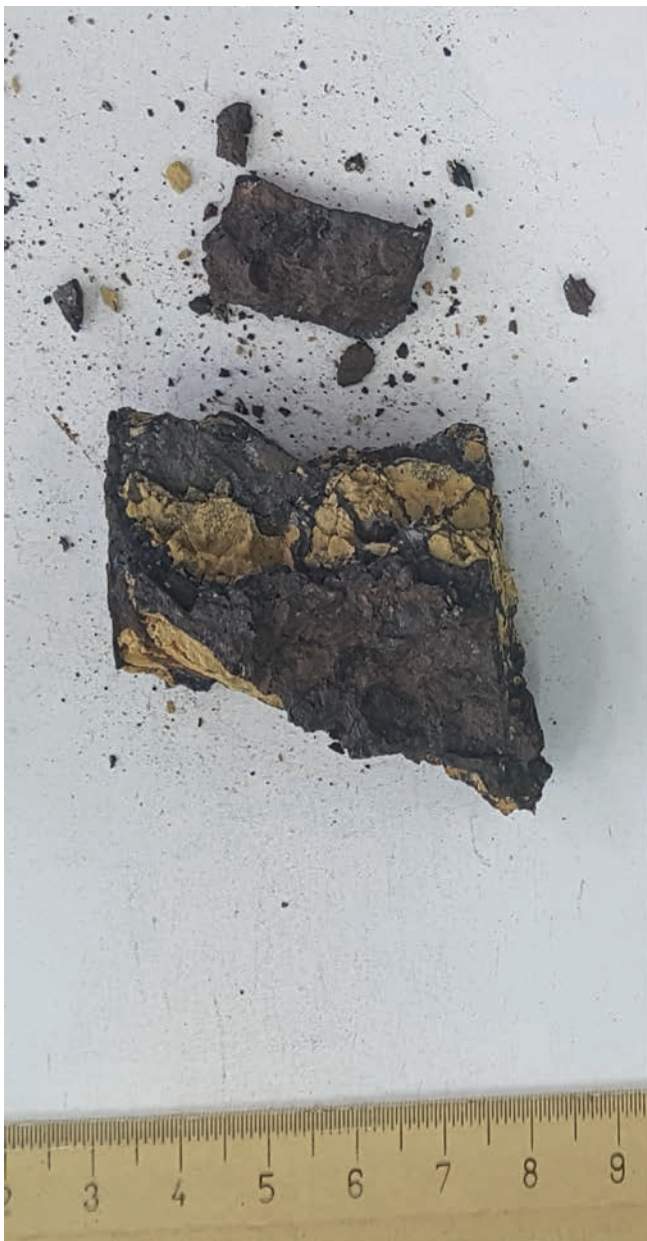
Fig. 5 - Dark manganese crusts on a claystone (sample V16A).
