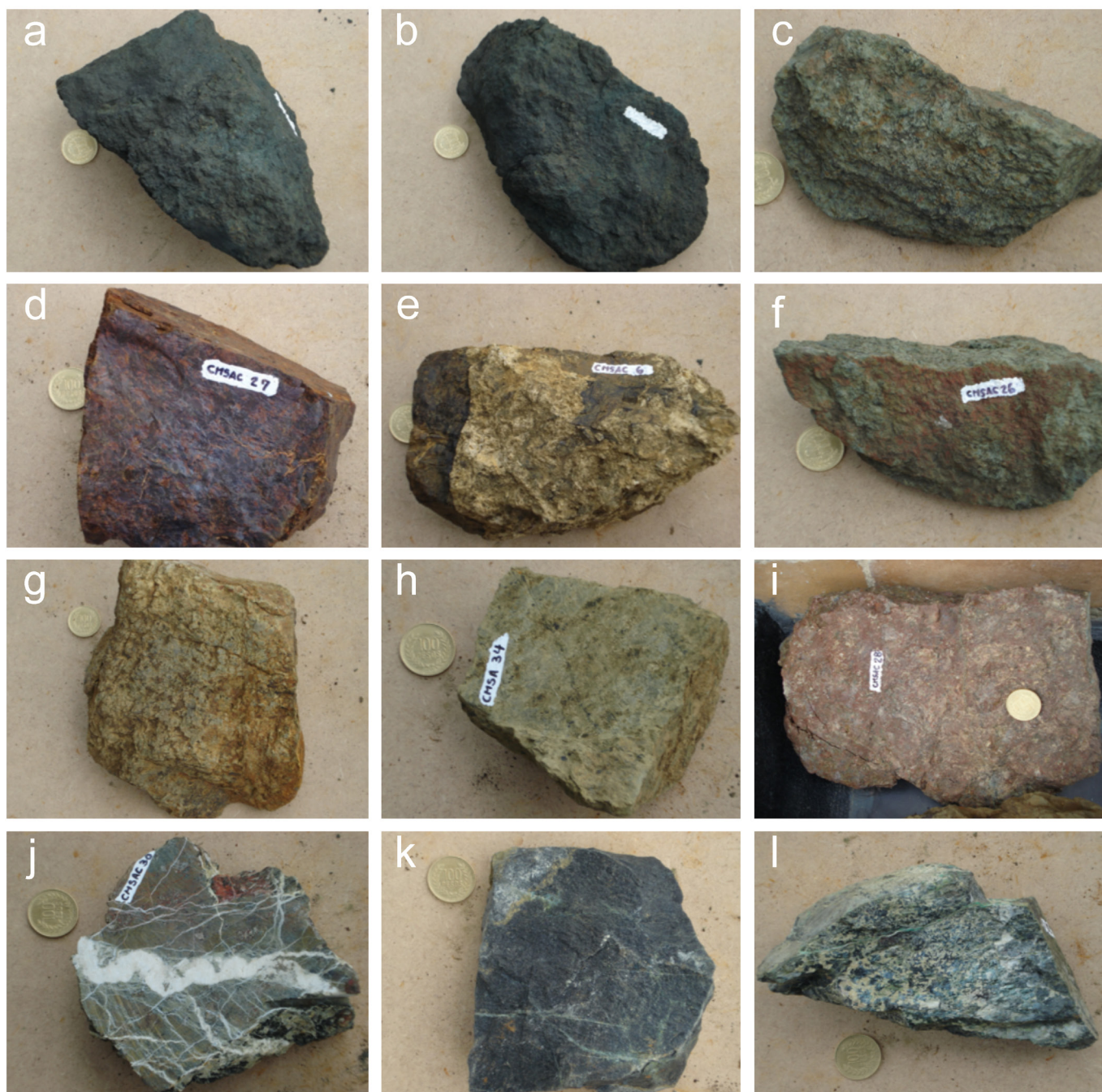
Fig. 3 - Hand samples collected from the Cerro Matoso deposit at Pit-1. a,b) Black mudstone facies II. C,f) Black mudstone facies II. D) Listvenite variety B, characterized by a purple color. e) Listvenite variety, characterized by brecciated texture with high silica/siderite vein content. g) Low-Mg green sapolite. h) High-Mg green sapolite. i) Sapolitized peridotite. j) Magnesite and silica veins in peridotite. k) Fresh peridotite. l) Serpentinized peridotite.
