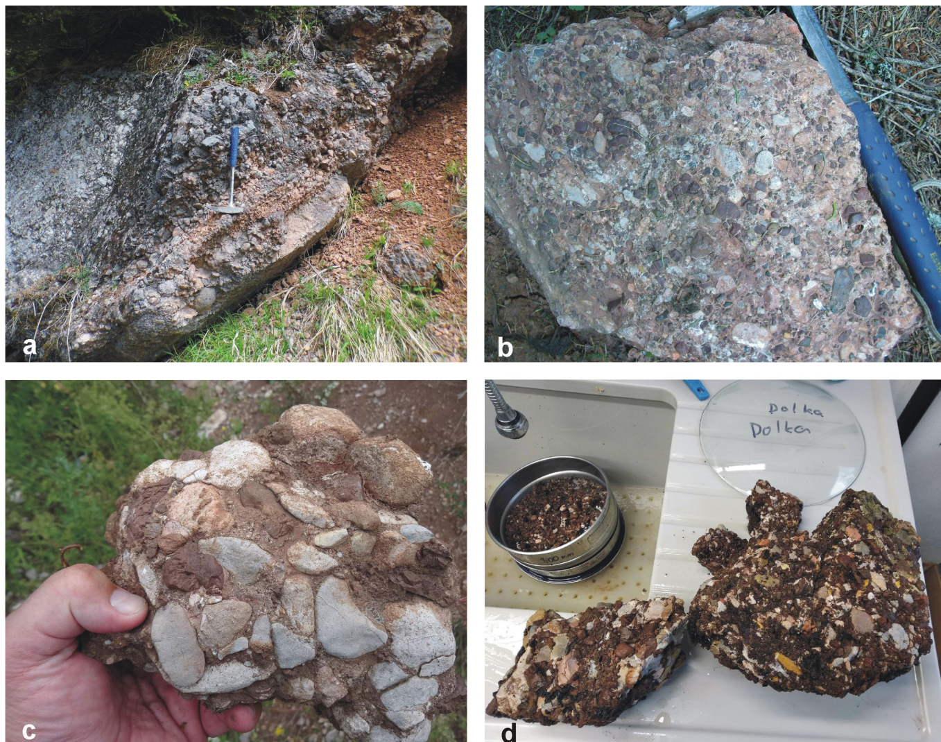
Fig. 2 - Examples of the studied conglomerates. a – One of the classical outcrops in a roadcut near the railway station (DLJ2 sampling site) showing conglomerate with limestone-dominated pebbles. b – Ostrá skala sample showing increased content of ophiolitic pebbles (red and green). c – Part of the DLJ1 sample showing limestone-dominated pebbles. d – Part of the Dolka sample during the laboratory dissolution process. The pebbles are mostly formed by ophiolitic material. However, a relatively low number of Cr-spinels extracted from the pebbles indicates that most of the ophiolitic pebbles were radiolarites, or magmatic rocks that did not contain Cr-spinels.
